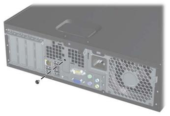
Figure 6-1 Removing the Smart Cover Lock Screw
